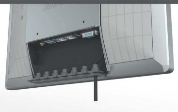
An important novelty is also innovative cable management, so that the user can easily and at any time reach the connectors, connect only the cable that he really needs and that the cable connection has IP protection.
